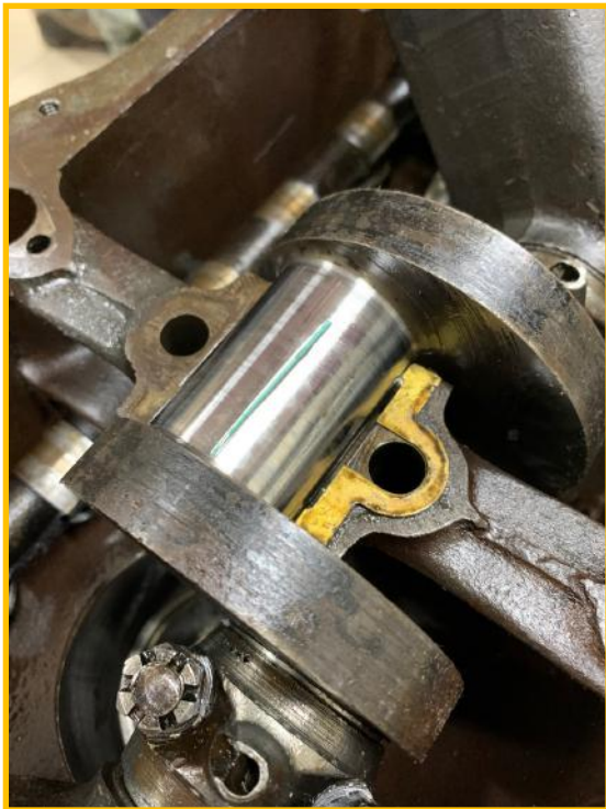
Center main with Plasti Gauge (note the blue line) ready to be checked.
