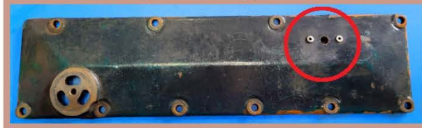
1929-1931 Valve Cover (side plate) with a drilled and tapped hole and crude riveted aluminum baffle installed inside. This hole is now my new fresh air inlet (J).
