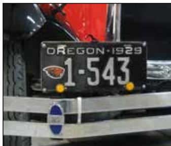
(Note: I have tried other years of the early V-8 Fords, and they do not fit the curve of the bumper bracket and they are not the height needed to place the license plate above the bumper. Additionally, please note that the 1939–1941 standard license plate bracket also does not fit correctly, so use the bracket from a deluxe passenger car.)
