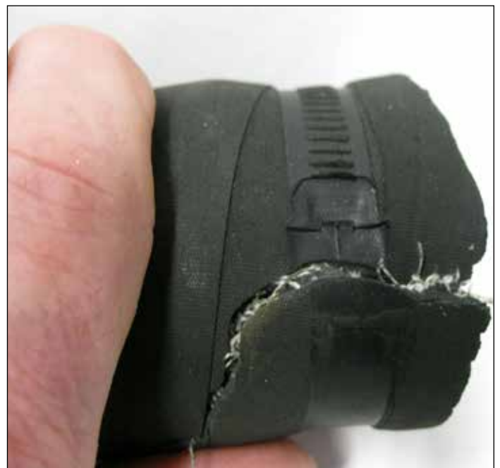
Photo 2: On the bottom side of the hose I found a two-inch-long tear.
