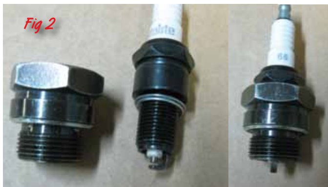
It is a good idea to use modern 14mm spark plugs with compression ratios above 5.5 to 1. This is easily done using spark plug adapter sets A-12405-ADP or A-12405-DAP.
