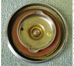
vent hole will be blocked off and the vacuum thing will happen. When you remove the cap you are liable to hear a "Whoosh" sound as air rushes into the tank to equalize the vacuum.
