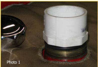
When I refuel my A's I use a drip bib (photo 1) which my wife made using a scrap piece of Naugahyde upholstery and left over fender welting. Next I insert my gas tank extension (photo 2) into the Model A fuel tank.
